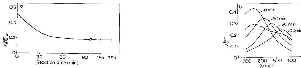
Fig. 2. Conversion of amylose to phytoglycogen by the 'branching enzyme'. Protein, 10 \mu g; amylose, 0.2 mg; buffer, 10 mM phosphate - 1 mM EDTA, pH 7.6, 3.0 ml. Incubation in duplicate at 30° under toluene vapor. Sample volumes of 0.2 ml were withdrawn at the times indicated and added to 1.2 ml of I 2 -KI reagent (a) or 1.2 ml of CaCl 2 -I 2 reagent (b). ( A_{660}^{1\text{ cm}} ) values were obtained on a Beckman DU, spectra on a Cary recording spectrophotometer. The spectrum of the CaCl 2 -I 2 complex of an equal mixture by weight of amylose and phytoglycogen, ○ — — — ○, is also presented in (b).
